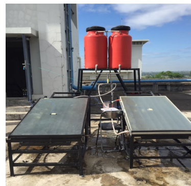
Fig. 2. SWH system using V-shaped absorber plate: on the left, with PCM storage and on the right, without PCM storage
